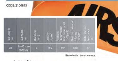
Laminate or Timber Floating Floor IXPE Closed-Cell Foam
