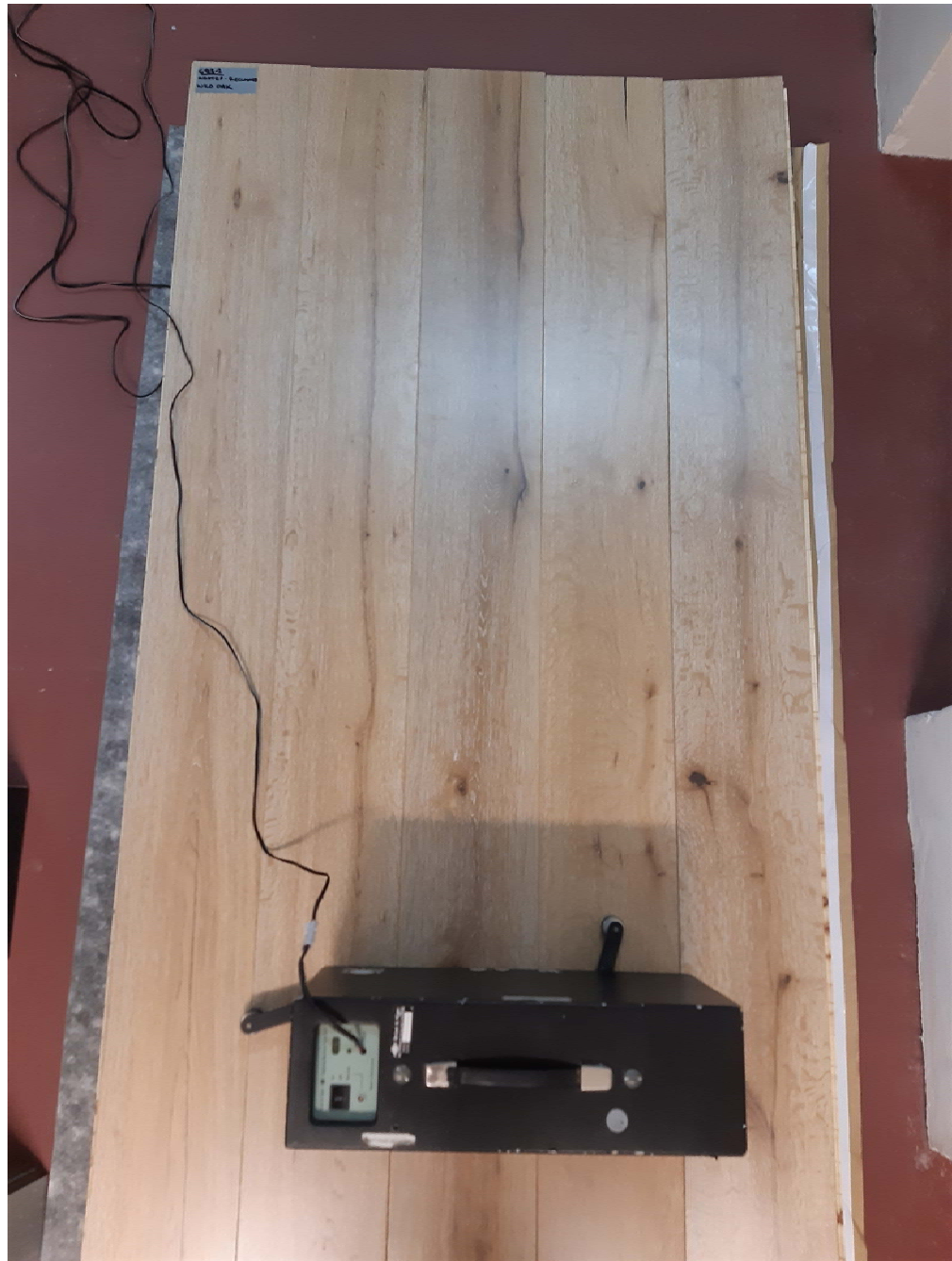
Figure 2. 14/3 mm "Reclaimed Wild Oak" engineered timber flooring product with 3 mm 'AcoustiStep' rubber underlay on top of base floor
