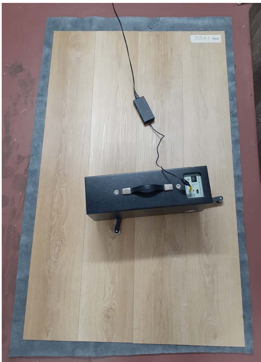
Figure 2. Image of testing configuration - '4 mm Vinyl Planks' with 'Helix' underlay on base floor
