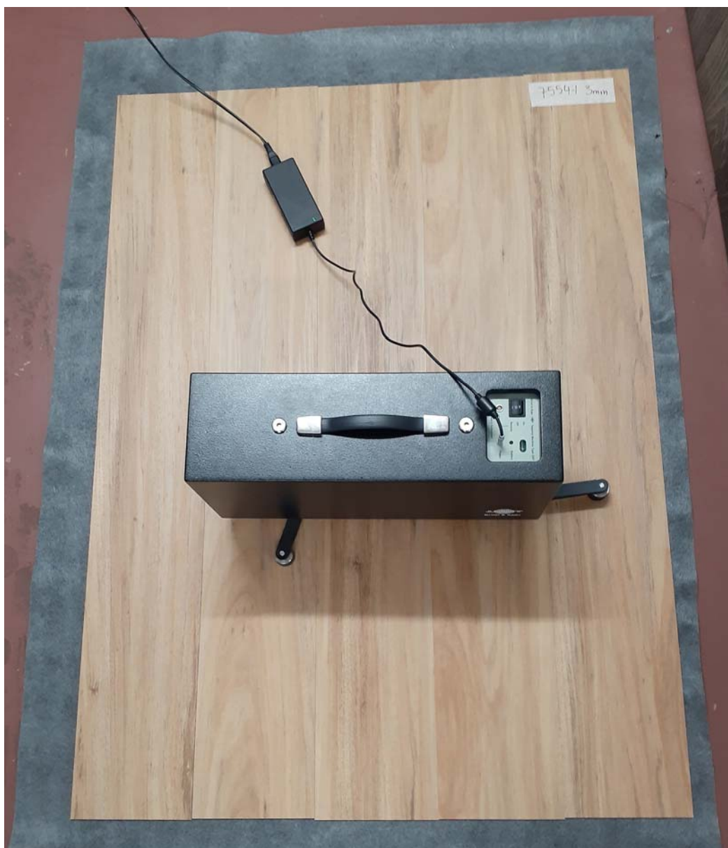
Figure 2. Image of testing configuration - '3 mm Vinyl Planks' with 'Helix' underlay on base floor
