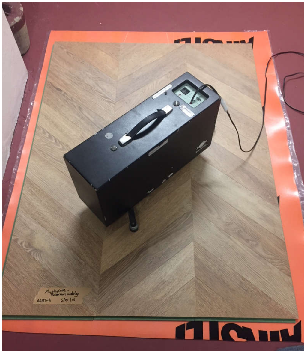
Figure 2. Image of testing configuration - 'Masterpieces' with 'Timbermax' underlay on base floor
