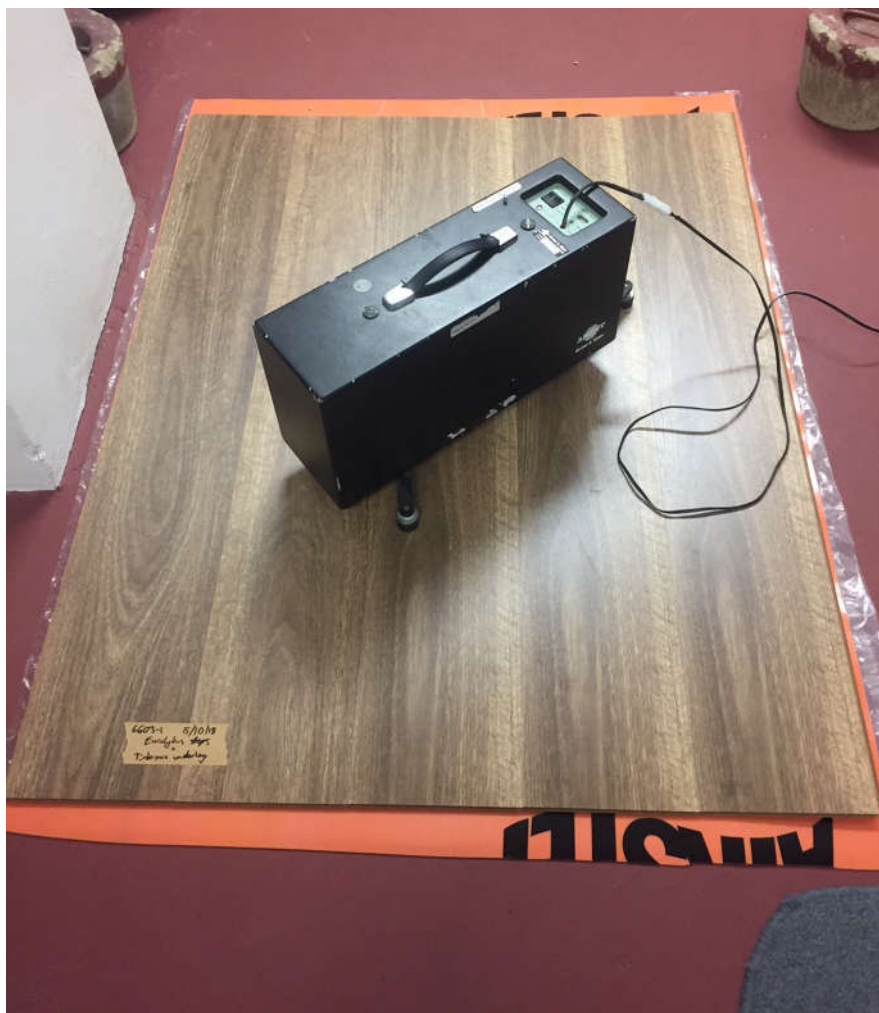
Figure 2. Image of testing configuration - 'Eucalyptus Steps' with 'Timbermax' underlay on base floor
