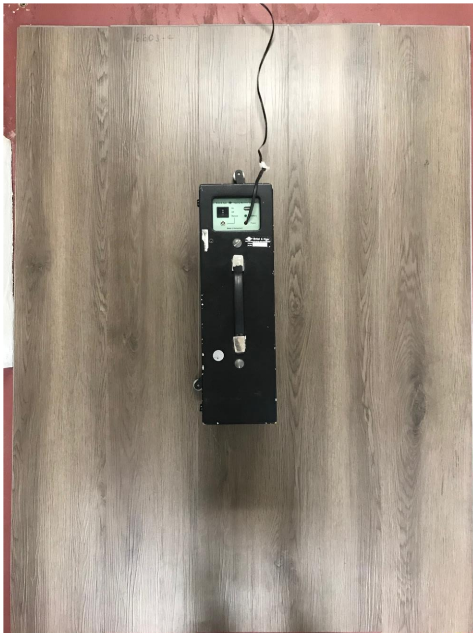
Figure 2. Image of testing configuration – Soleil “Multilayer Hybrid” flooring atop the base concrete floor
